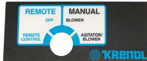
Identifies if machine is in remote mode, manual mode, or off position. In manual mode this switch operates machine. In remote mode the hand pendant operates machine. Each time machine cycle starts, an audible alarm warns the operator that the machine is about to come on.
